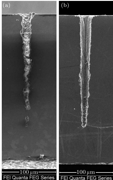
Fig. 1. Morphology of silicon micro-hole: (a) the LISC zone, (b) after selective chemical etching.
