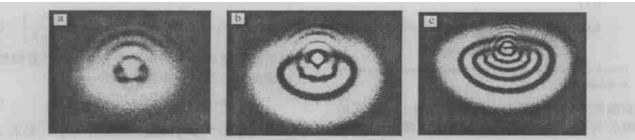
Fig.4 Diffraction rings induced by dominant thermo-optic effect a- P\approx 3.36\text{mW} b- P\approx 6.02\text{mW} c- P\approx 9.34\text{mW}
